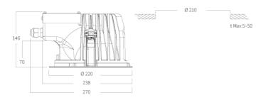
Efficient, robust downlight suitable for various application areas with several luminous fluxes and distribution angles.
